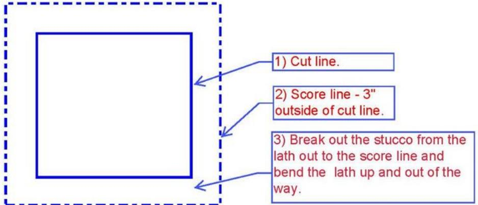
Diagram 2 – Placing the Jumbo-Tex 60 in the patch area
