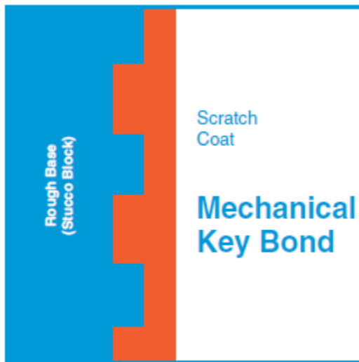
Figure 1 – Mechanical key bond
